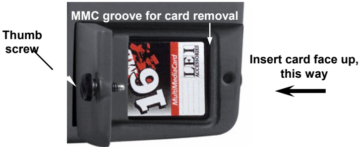
Memory card compartment with a 16 MB MMC card installed.
